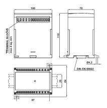
The unit is intended for mounting on a standard DIN rail. Avoid mounting the unit where there is excessive vibration; in excessive direct sunlight; or outside a reasonably stable ambient temperature of -10 to +45°C.
